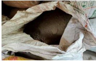
Gambar 2. Fly ash (Ridzeki, F., dkk, 2024)
